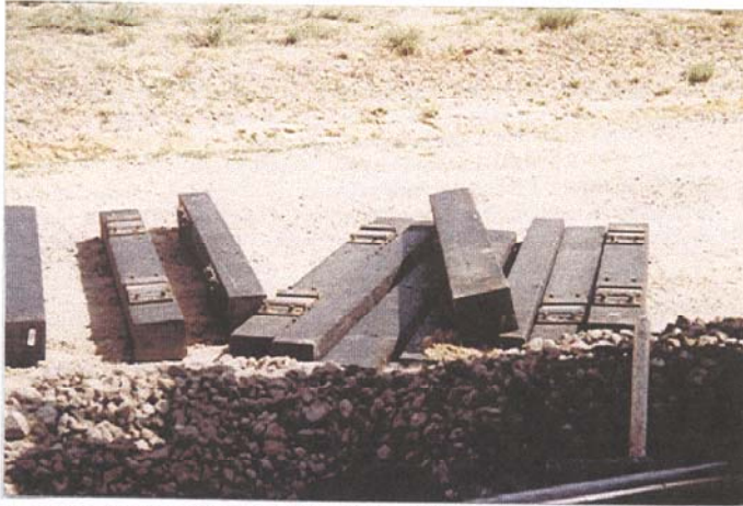
Figure 2- Recycled Plastic Railroad Ties Prior to Installation at AAR's FAST Track in Pueblo, CO.
