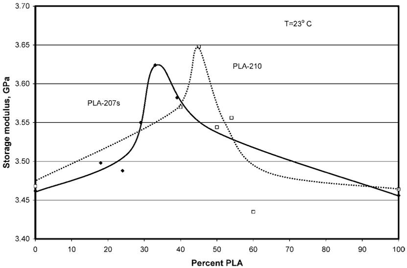
**Figure 3.** Storage modulus by DMA for PLLA/PMMA blends. Regions of phase co-continuity are shown by maxima.
