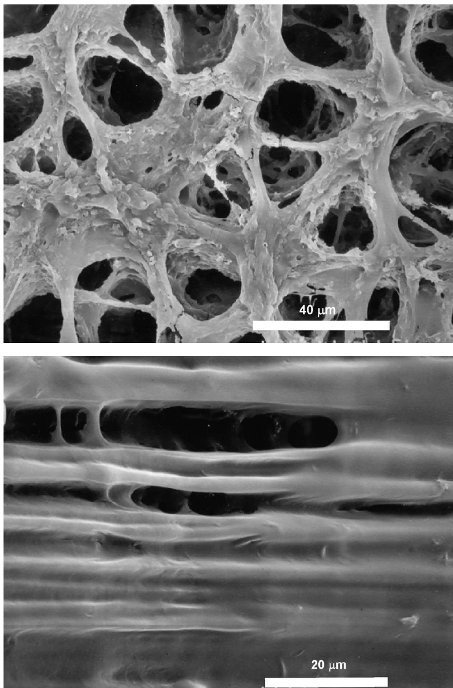
**Figure 1.** (Top) 28/72% (v/v) PLLA/PMMA composite: DMF etched, sectioned perpendicular to extrusion axis. (Bottom) 28/72% (v/v) PLLA/PMMA composite: DMF etched, sectioned parallel to extrusion axis.
