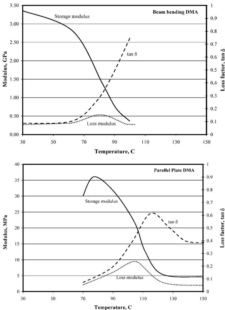
**Figure 2.** (Top) Flexural DMA data on PLA L207S/PMMA composite (28 vol% PLLA), illustrating low-temperature transitions. (Bottom) Parallel-plate DMA data on PLA L207S/PMMA composite (28 vol% PLLA), illustrating high-temperature transitions.
