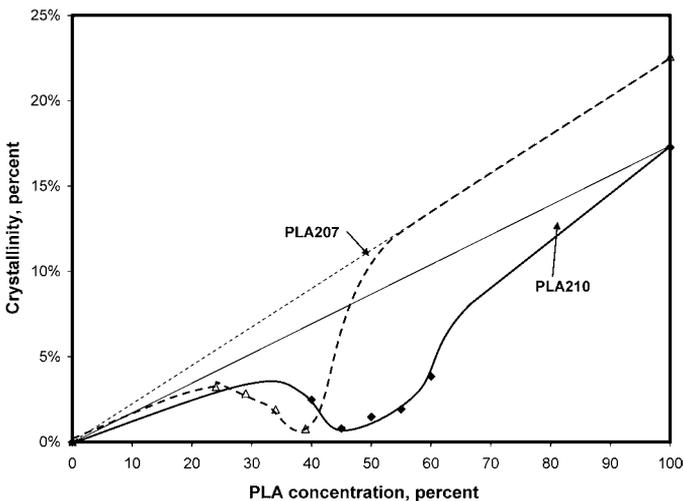
**Figure 7.** PLLA crystallinity versus percentage of the blend. Straight lines show expected behavior based on crystallinity of pure blend compositions.
