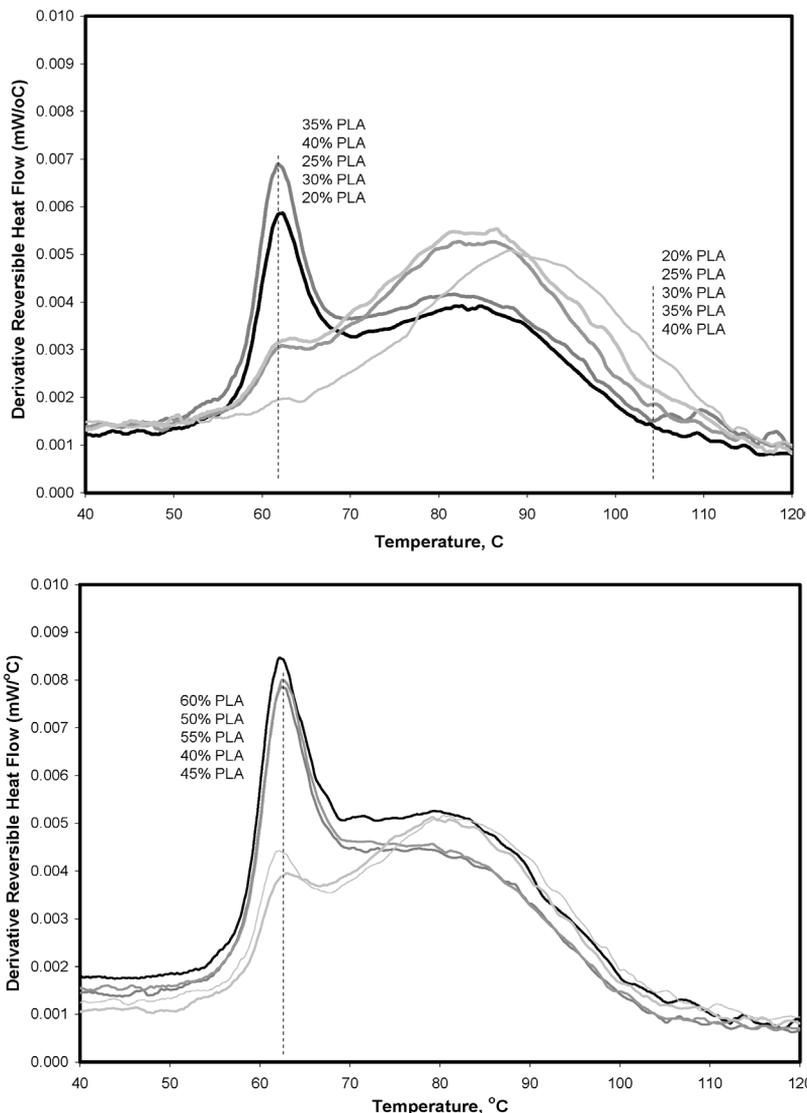
**Figure 4.** (Top) Derivative of reversing heat flow from MDSC analysis of PLA L207S/PMMA blends. (Bottom) Derivative of reversing heat flow from MDSC analysis of PLA L210/PMMA blends.
