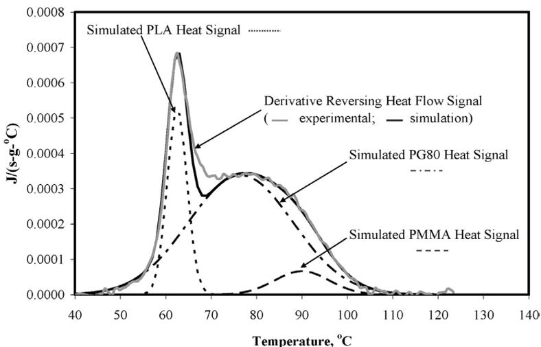
**Figure 5.** Example of DSC curve deconvolution using normal distribution function simulations of constituent  $T_g$  derivative heat signals.
