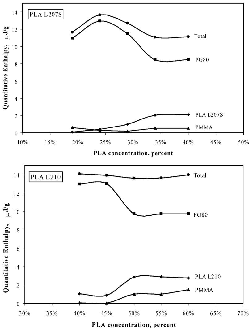
**Figure 6.** (Top) Quantitative DSG data for PLA L207S/PMMA blends illustrating PG80 maximum near the co-continuous composition. (Bottom) Quantitative DSG data for PLA L210/PMMA blends illustrating PG80 maximum near the co-continuous composition.
