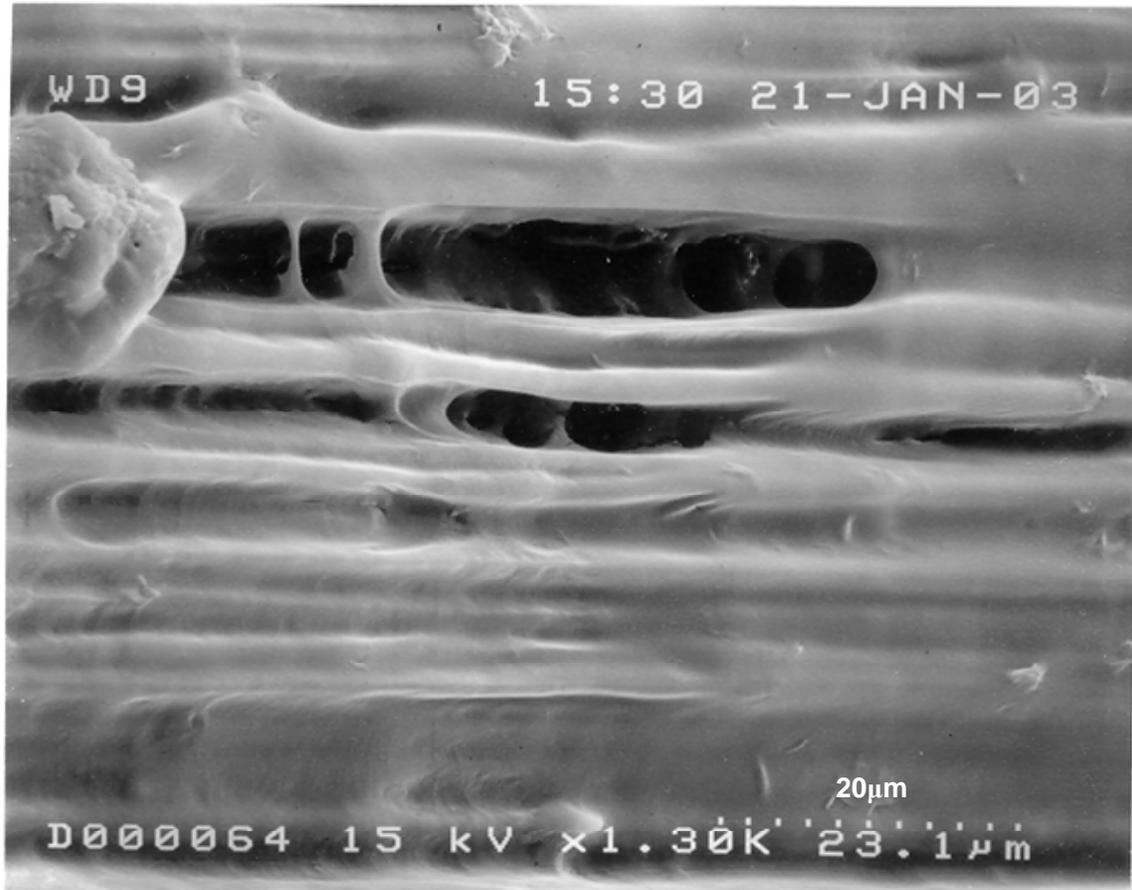
**Figure 2b:** SEM image of PLLA/PMMA immiscible blend composites etched to show architecture of blend after transient phase is removed. Sample sectioned parallel to extrusion axis.
