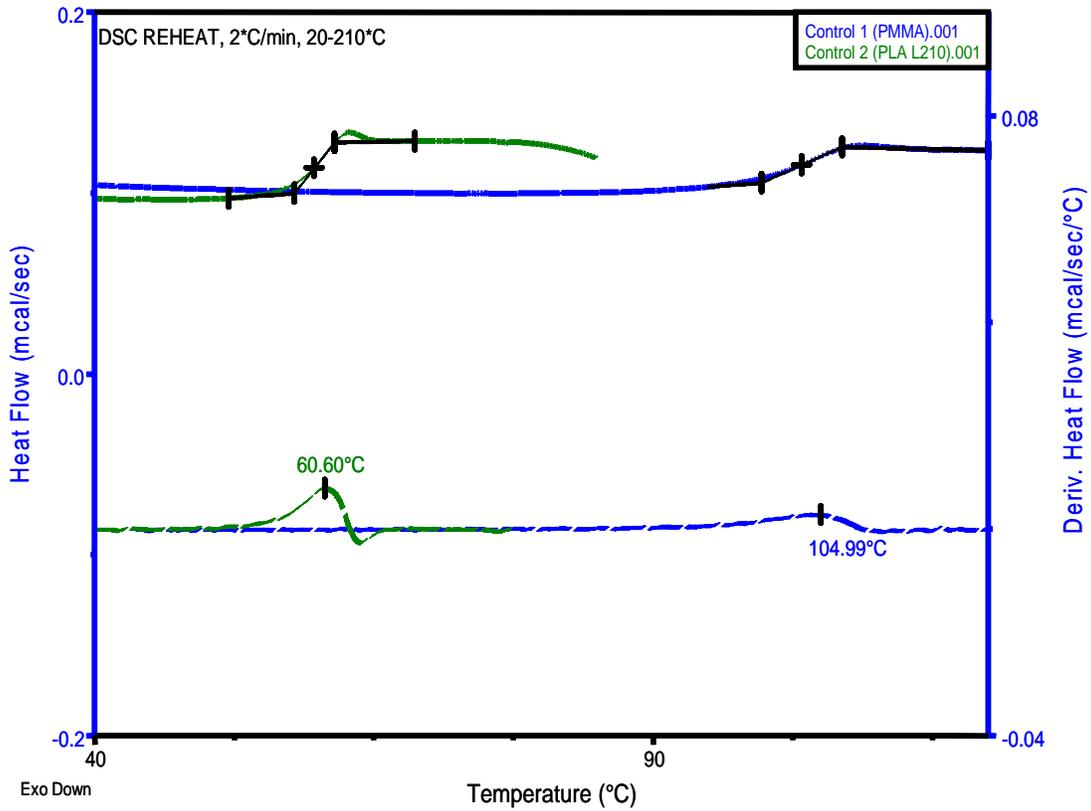
**Figure 4b:** DSC data for neat end-member polymers PLLA 210 and PMMA showing glass transitions for each.
