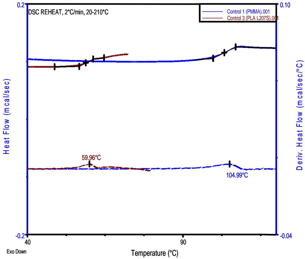
**Figure 4a:** DSC data for neat end-member polymers PLLA 207S and PMMA showing glass transitions for each.
