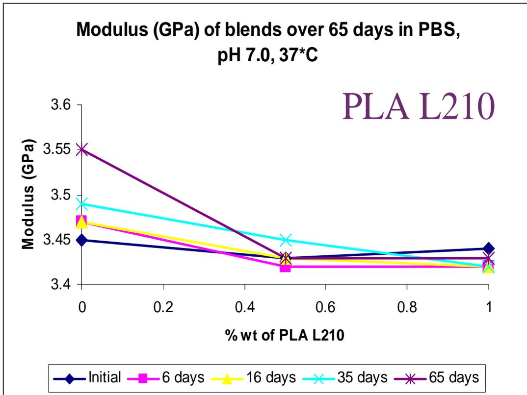
**Figure 7b:** Elastic modulus retention under aging in PBS at 37 °C for up to 65 days. Abscissa is weight fraction of PLLA 210 in PLLA/PMMA blend.
