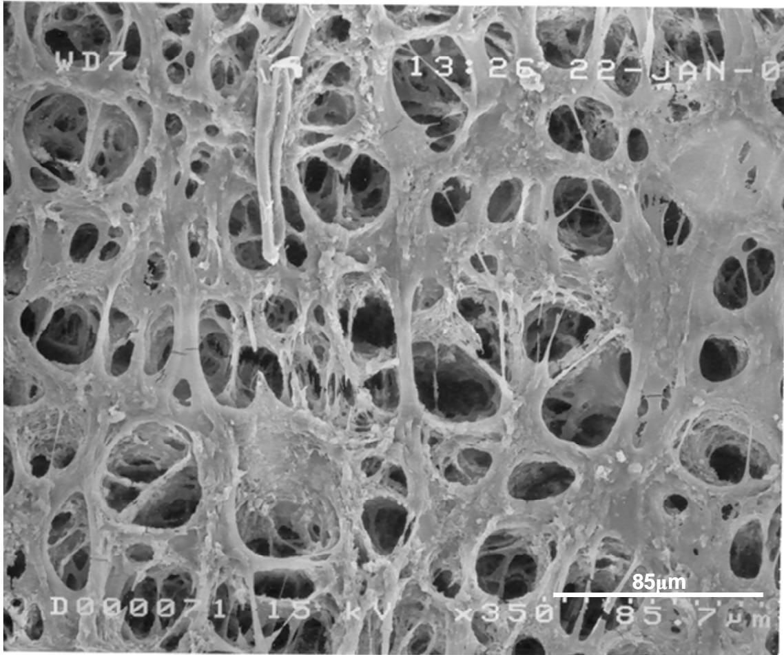
**Figure 2a:** SEM image of PLLA/PMMA immiscible blend composites etched to show architecture of blend after transient phase is removed. Sample sectioned perpendicular to extrusion axis.
