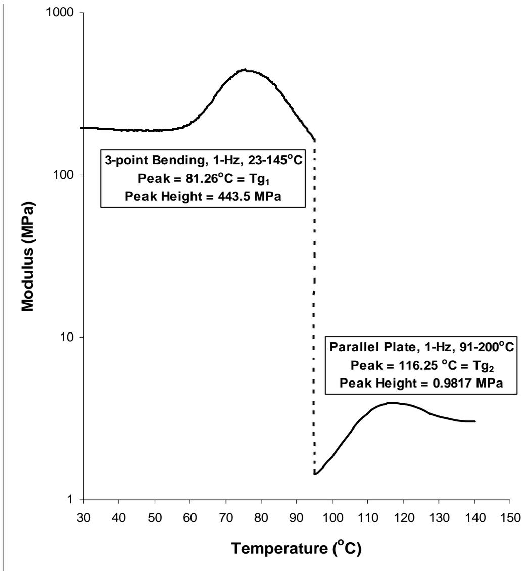
**Figure 3:** Two glass transitions observed in PLLA/PMMA blends by DMA. The low temperature  $T_g$  corresponds to PLLA and was measured by 3-point bending. The high temperature  $T_g$  was measured by parallel plate methods and corresponds to PMMA.
