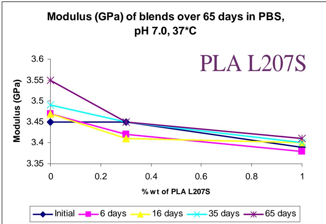
**Figure 7a:** Elastic modulus retention under aging in PBS at 37 °C for up to 65 days. Abscissa is weight fraction of PLLA 207S in PLLA/PMMA blend.
