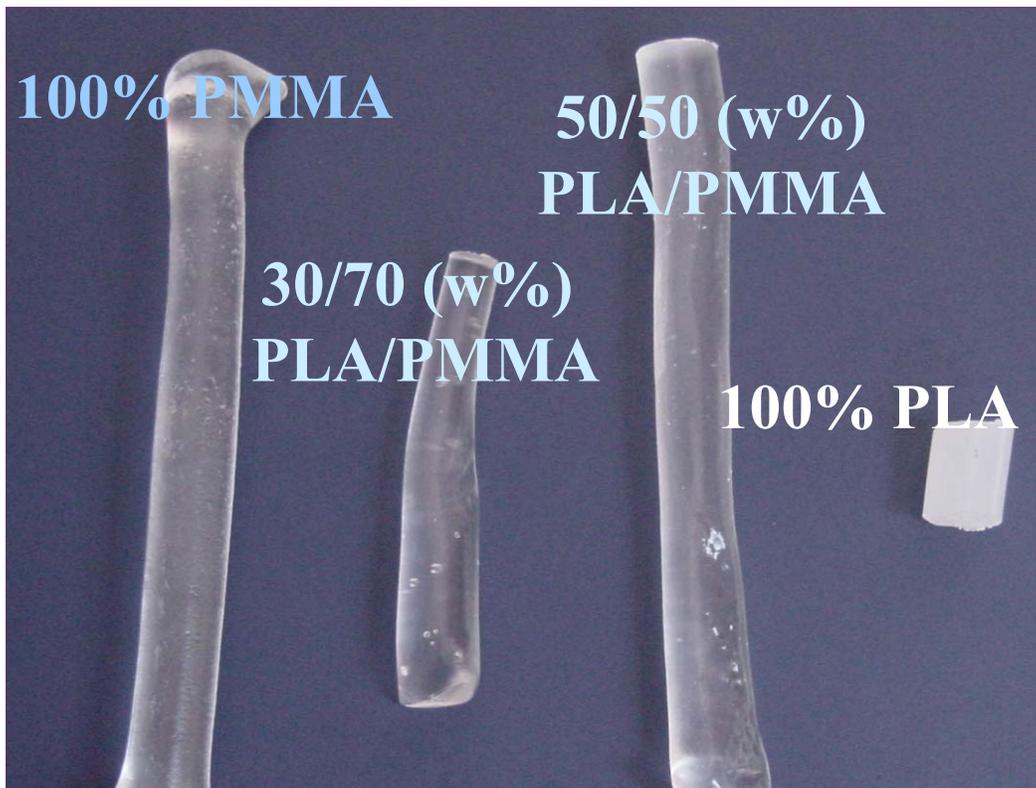
**Figure 1:** PLLA/PMMA immiscible blend composites illustrating optical clarity.
