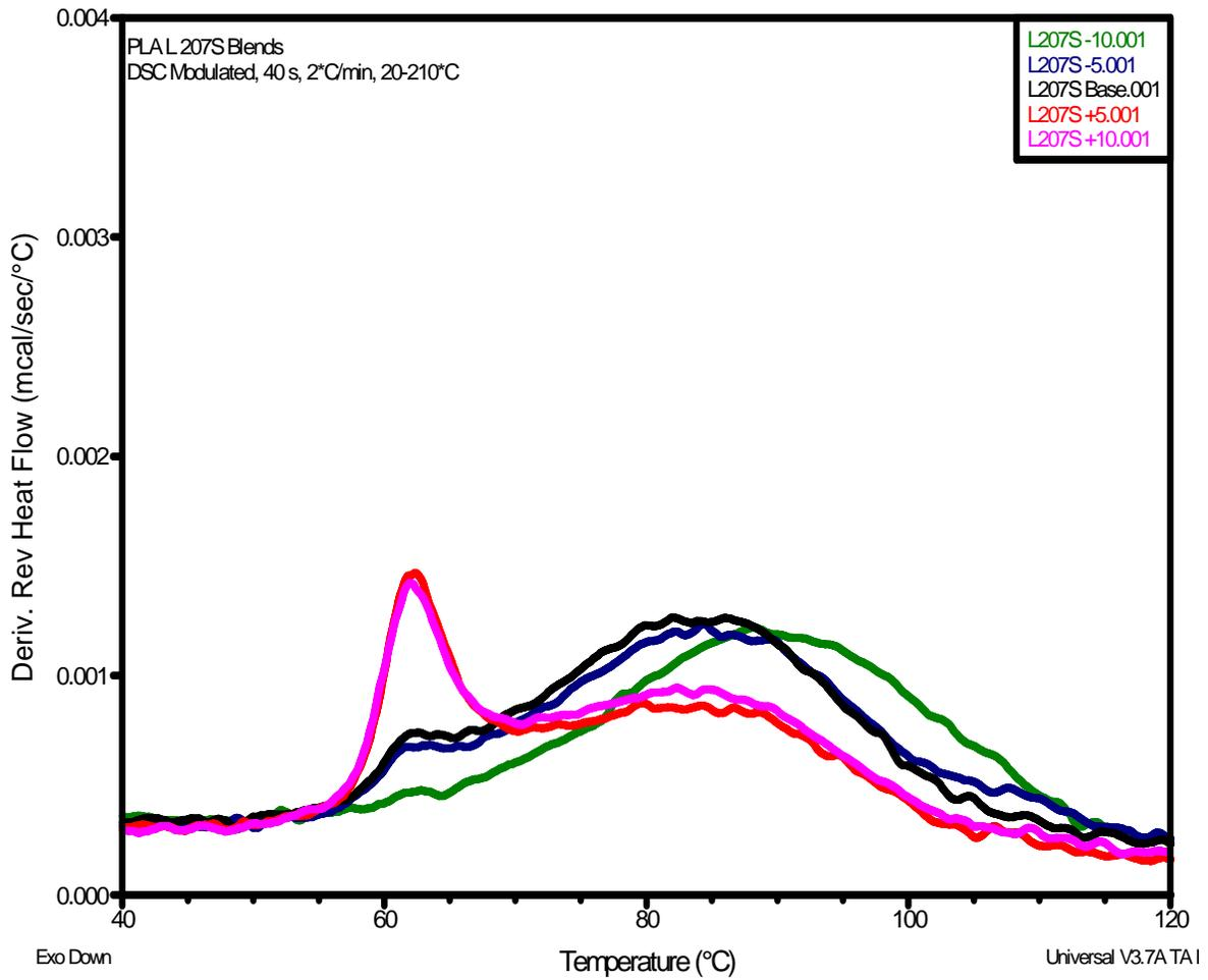
**Figure 5a:** DSC derivative heat flow profiles of PLLA/PMMA blends in the vicinity of the co-continuous composition for blends prepared with PLLA 207S
