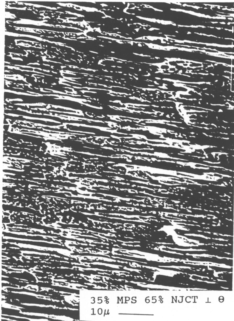
Figure 3: SEM Micrograph of 35/65 MPS/NJCT
