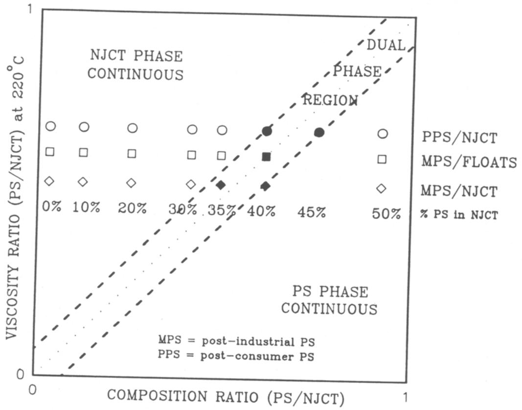
Figure 5: Plot of Viscosity Ratio Versus Composition Ratio for the Various PS/NJCT Materials Indicating the Dual Phase Compositions
