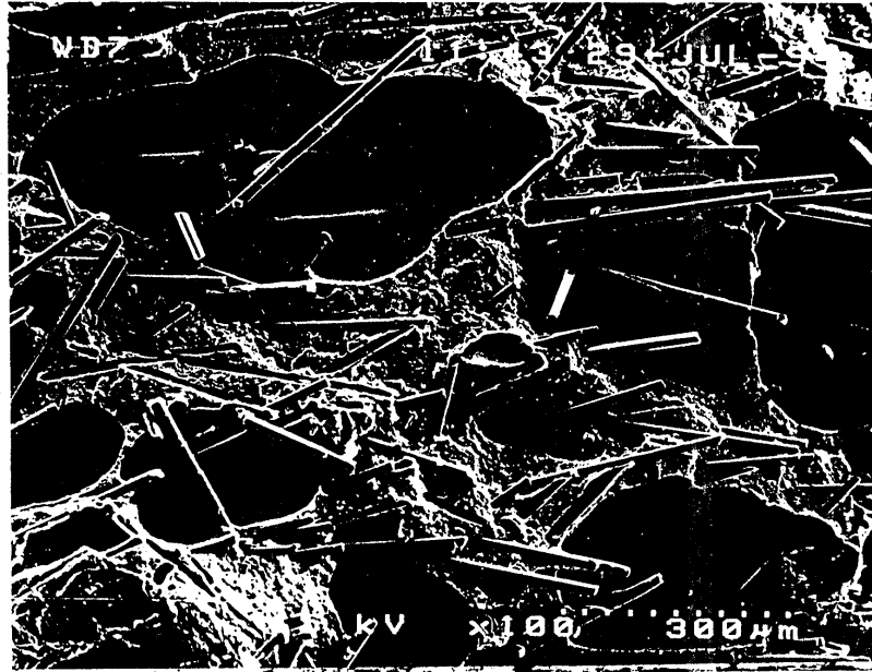
Figure 7: Scanning electron micrograph of material L, showing a 'log-jam' of oriented glass fibers in a porous polymeric matrix. The surface is parallel to the long axis of the lumber profile, running across the width of the photo.
