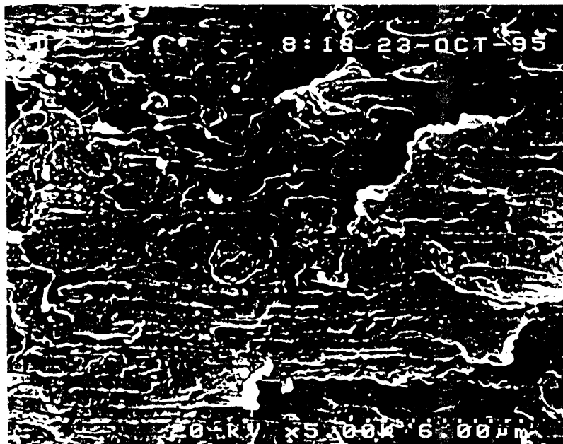
Figure 6: Scanning electron micrograph of material F. A highly oriented two-phase system is evident. The surface is parallel to the long axis of the lumber profile, running across the width of the photo.
